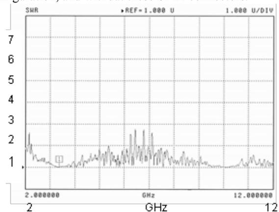
Fig. 6. Measured SWR for array with 0° scan.
