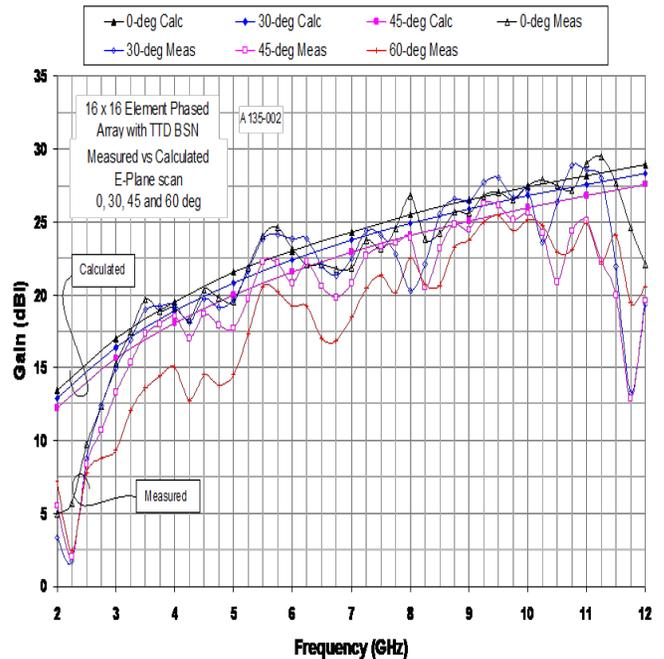
Fig. 10. Comparison of measured and simulated  $E$ -plane antenna gain over 2-12 GHz for scans at  $0^\circ$ ,  $-30^\circ$ ,  $-45^\circ$  and  $-60^\circ$  off broadside.
