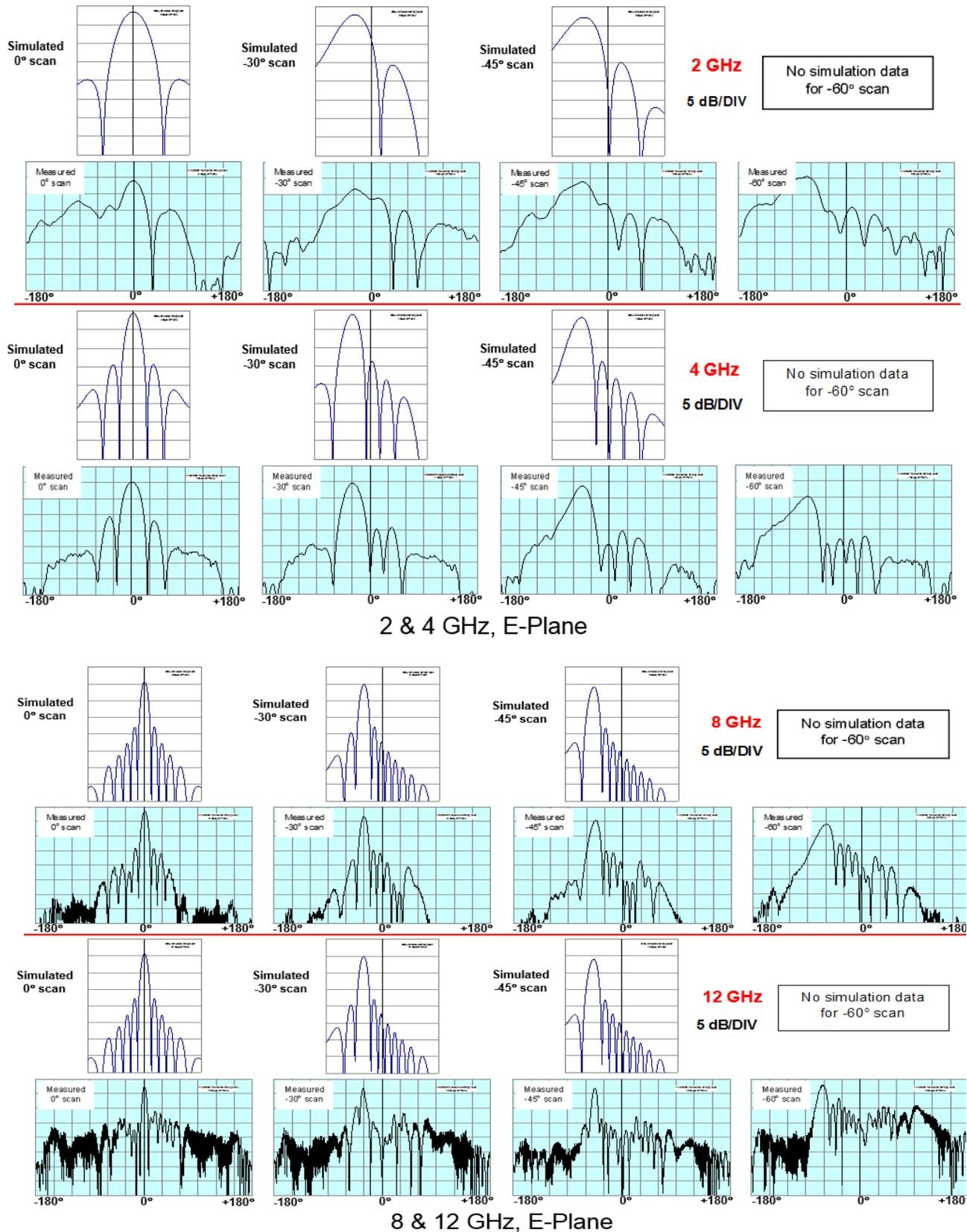
Fig. 8. Comparison of measured and simulated E-plane radiation patterns for scan at 0°, -30°, -45° and -60° off broadside at 2, 4, 8, and 12 GHz.
