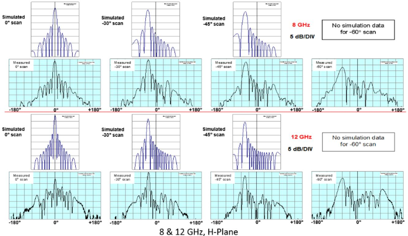
Fig. 7. Comparison of measured and simulated *H*-plane radiation patterns for scan at 0°, -30°, -45° and -60° off broadside at 2, 4, 8, and 12 GHz.
