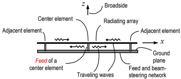
Fig. 3. Cross-sectional view around a center element of a TWAA.
