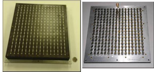
Fig. 1. Photograph of the TWAA in front and back views.
