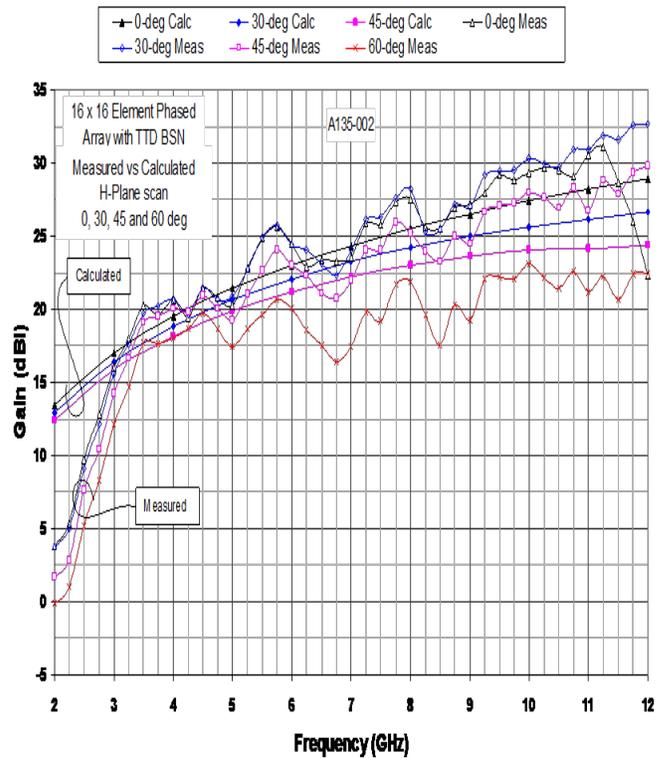
Fig. 9. Comparison of measured and simulated  $H$ -plane antenna gain over 2-12 GHz for scans at  $0^\circ$ ,  $-30^\circ$ ,  $-45^\circ$  and  $-60^\circ$  off broadside.
