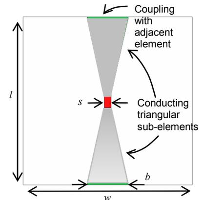
Fig. 2. Unit cell of planar TWA array with planar bowtie dipole element.
